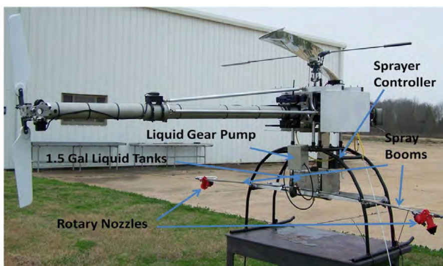
Figure 1. UAV helicopter spray system with spray system mounted on the undercarriage (modified from Huang et al., 2013)
